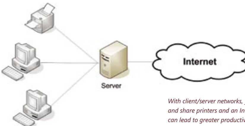
*With client/server networks, you can centralize files and share printers and an Internet connection, which can lead to greater productivity and cost savings.*
